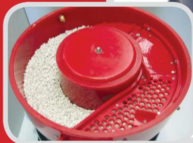
Designed and manufactured in our factory in Melbourne and offered with a 5 year warranty the Technovibe range offers entry level pricing with a variety of upgradeable options (see over page). This machine is a full industrial duty bowl machine capable of performing all the usual surface finishing operations using a
