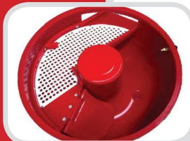
Designed and manufactured in our factory in Melbourne and offered with a 5 year warranty the Technovibe DR range offers entry level pricing with a variety of upgradeable options. (see over page) This machine is a full industrial duty bowl machine capable of performing all the usual surface finishing operations using a variety of medias and chemicals. From vigorous deburring to gentle state of the art polishing. The DR series also has BV Products unique
